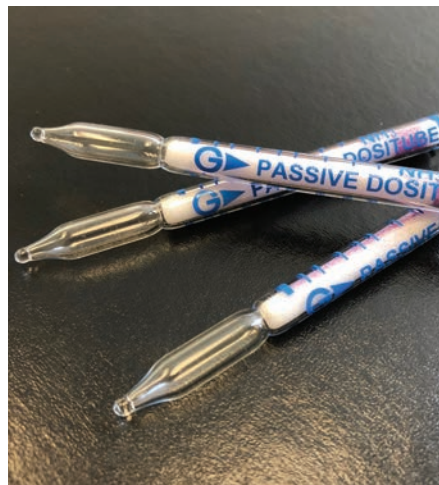
▲ Passive colorimetric ammonia dosimeters for measuring ammonia volatilization rate in the field.
