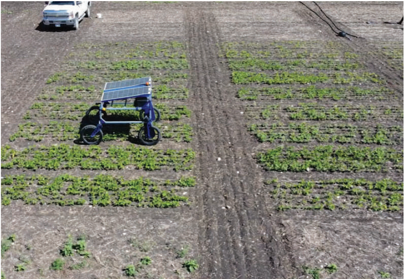
TerraByte's data rover gathers field images and measurements, helping train AI models for weed detection, disease identification and crop analysis. Image courtesy Michael Beck.
