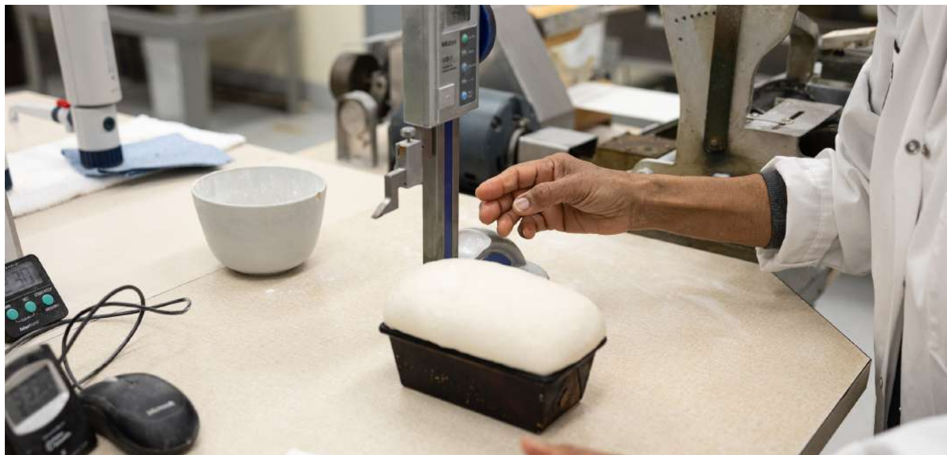
ABOVE: Bread dough after proofing. LEFT: Bread loaf as part of wheat end-use quality testing inside a VolScan Profiler, which measures the volume, density and dimensional profiles of bread and bakery products. Images courtesy of the Canadian Grain Commission.
