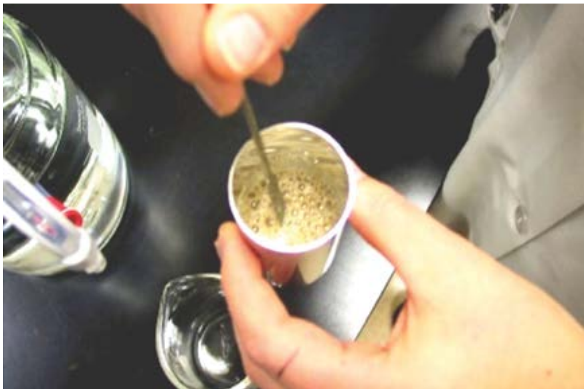
Figure 1. Preparation of ground barley grain and water mixture for RVA analysis. Photo courtesy of Dr. Marta Izydorczyk, Canadian Grain Commission.
