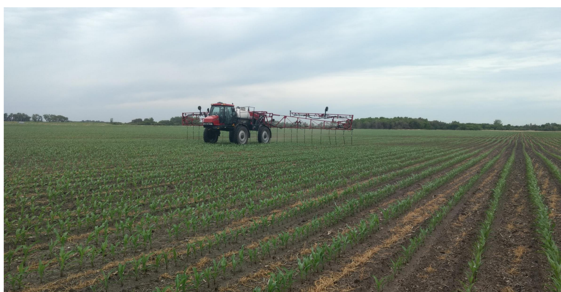
Figure 4 – Sidedress application of UAN with custom y-drop hoses on strip-tilled land at one site – June 14, 2018
