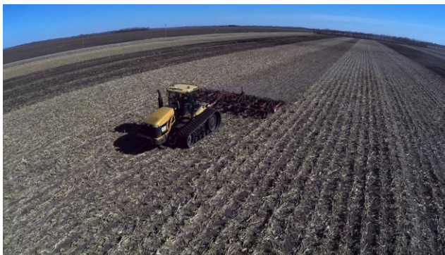
Figure 3: Vertical till low disturbance (0° disc angle). Some soil movement is observable when compared to the area of undisturbed soil to the right. Surface residue coverage after two passes was 65%. Photo Credit: Patrick A. Walther
