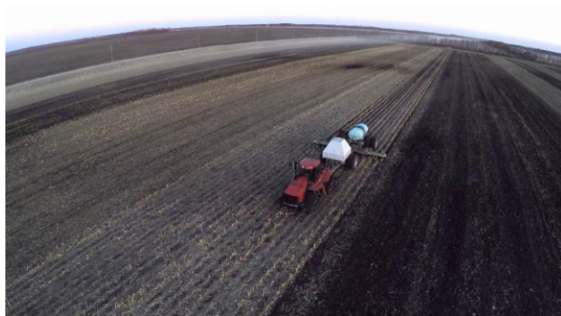
Figure 4: Strip till uses tillage in only a small strip zone and leaves the area in-between the shanks untilled. This unit consists of two fertilizer carts for granular (white) and liquid (turquoise) fertilizer placement. Surface residue coverage after two passes was 4% in the strip, 95% between the strips and 63% when analysed over the entire area. Photo Credit: Patrick A. Walther
