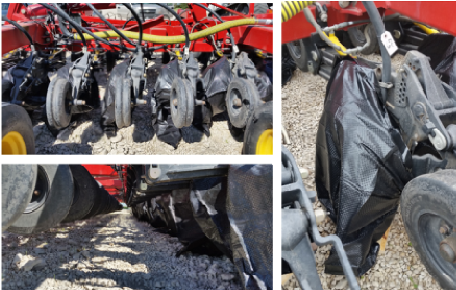
Figure 8. Bags were placed around each opener to collect product during each repetition.
