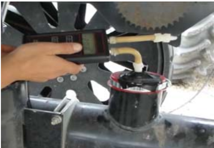
Figure 5. Static pressuring monitoring on the Bourgault set-up near the fan.
