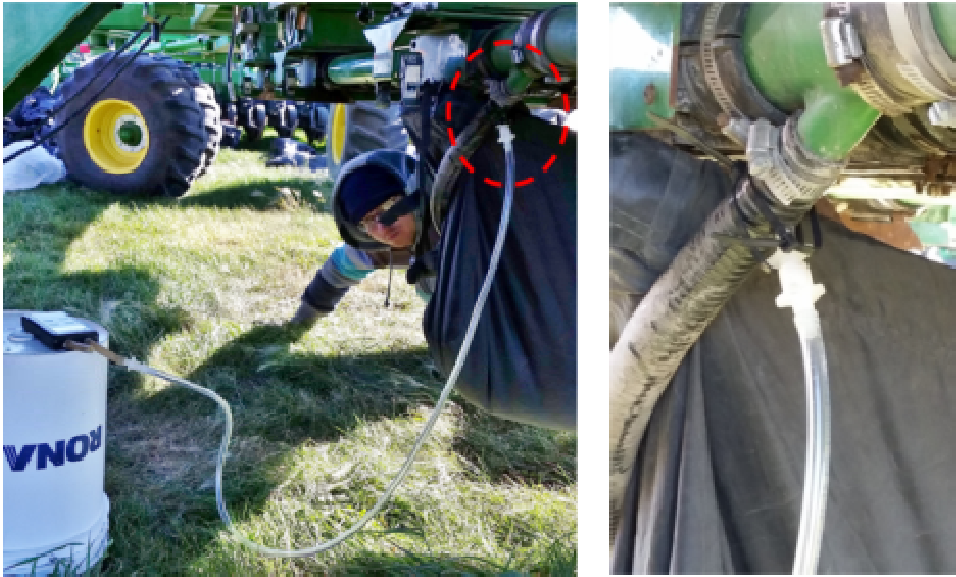
Figure 4. Static pressure monitoring on the John Deere set-up near the fan.
