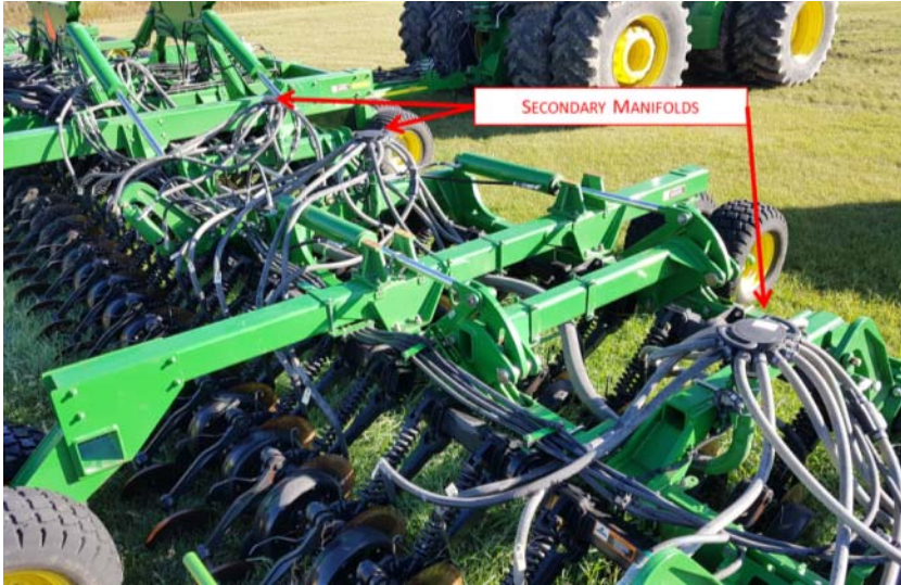
Figure 2. John Deere set-up with locations of secondary manifolds.
