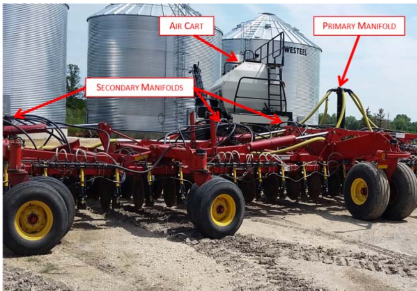
Figure 1. Bourgault set-up with locations of secondary manifolds.
